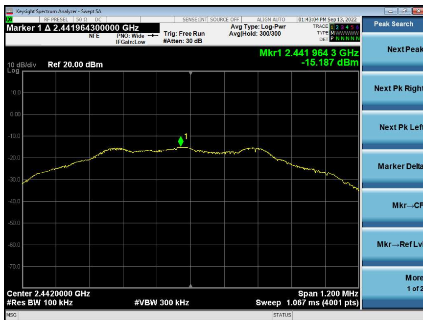
Figure Tr17.4: Partially corrected power spectral density data for Bluetooth Low Energy, 2442 MHz
