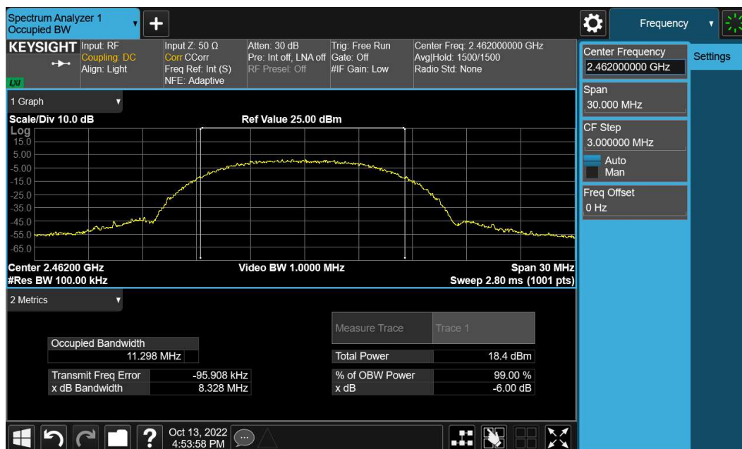
Figure TR46.3: DTS bandwidth data for 802.11b 11 Mbps at channel 11
