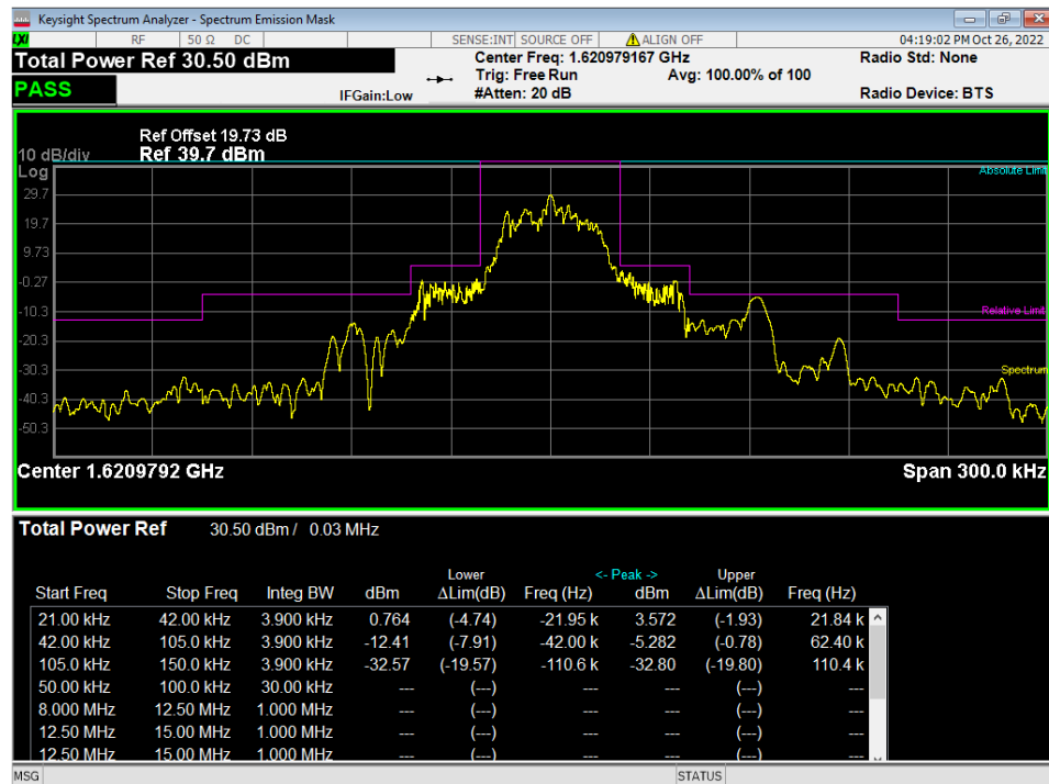
Figure 6 – Part 25.202(f) Mask, Transmitting at 1620.979167 MHz
