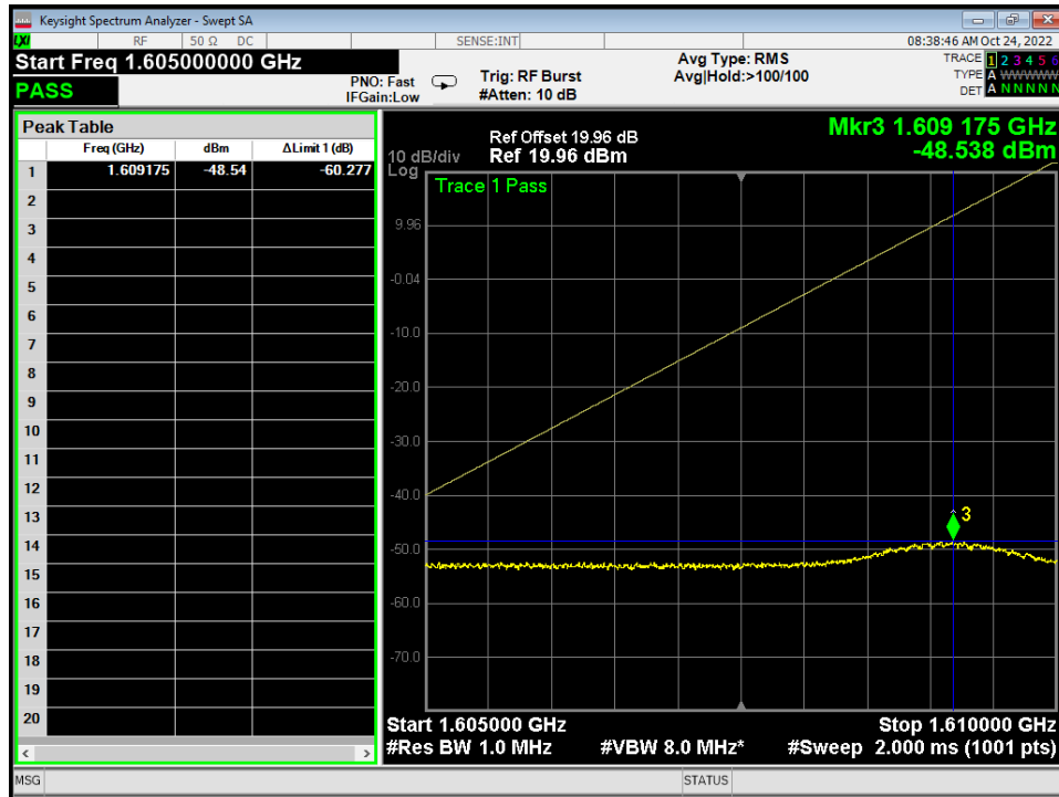
Figure 13 – Part 25.216(g), Transmitting at 1625.979167 MHz, Conducted Measurement
