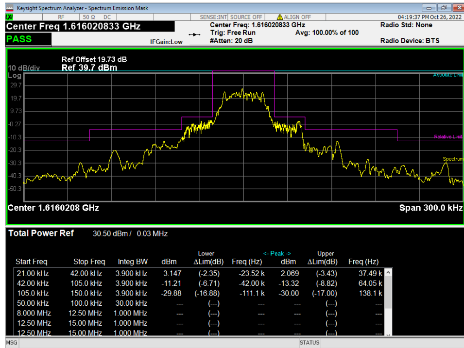
Figure 5 – Part 25.202(f) Mask, Transmitting at 1616.020833 MHz
