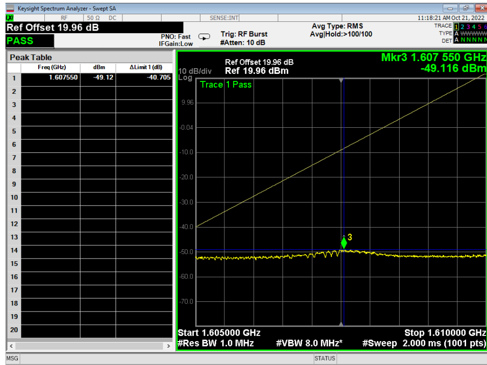
Figure 11 – Part 25.216(g), Transmitting at 1616.020833 MHz, Conducted Measurement
