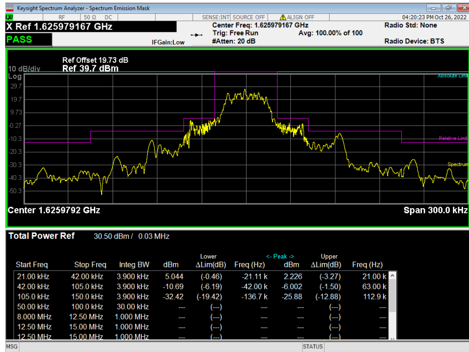
Figure 7 – Part 25.202(f) Mask, Transmitting at 1625.979167 MHz
