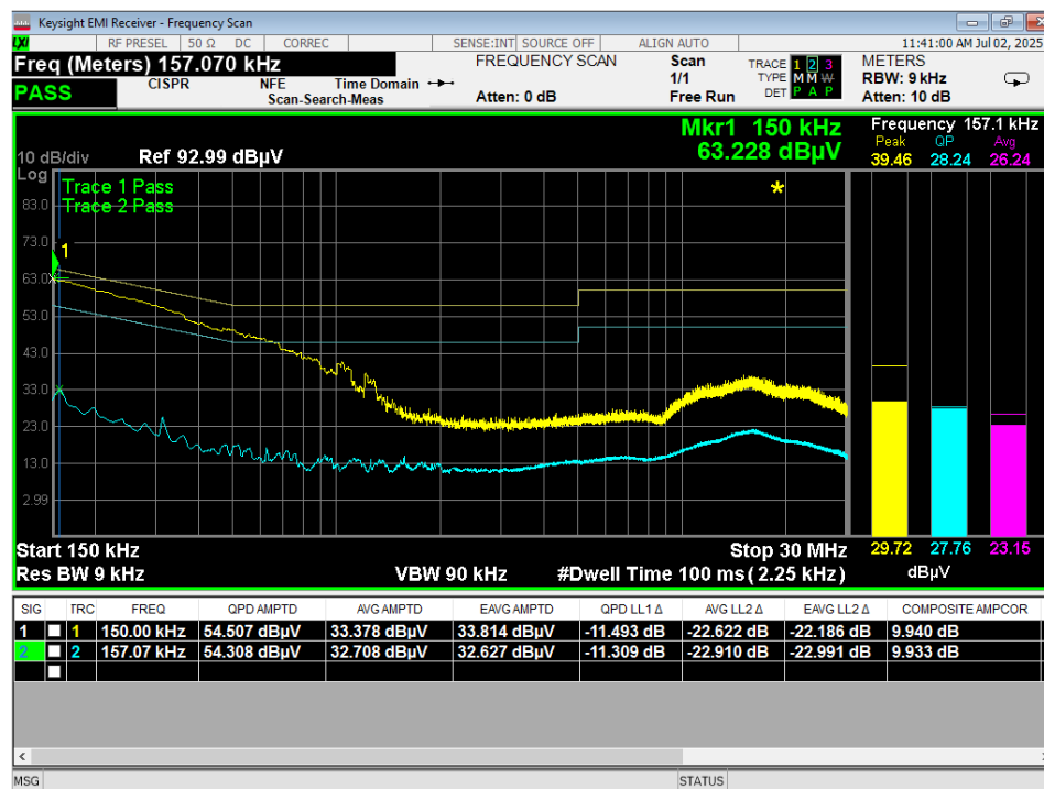
Figure 20 – Conducted Emissions Plot, charging via USB-C, IDLE, Line
