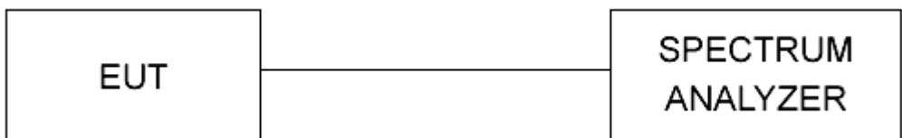
Figure 1 - Bandwidth Measurements Test Setup
