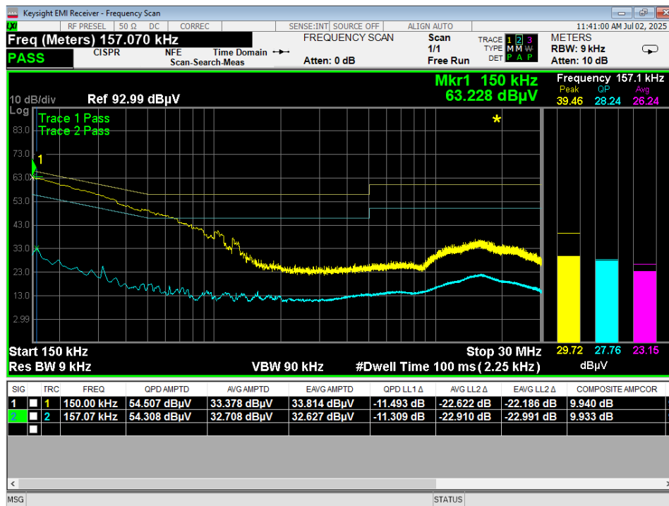
Figure 27 – Conducted Emissions Plot, charging via USB-C, IDLE, Line
