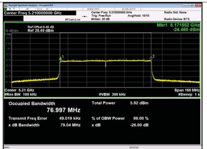
IEEE 802.11ax\_80\_Channel 42\_80MHz\_Antenna
