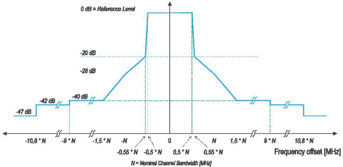
NOTE: dBc is the spectral density relative to the maximum spectral power density of the transmitted signal.
