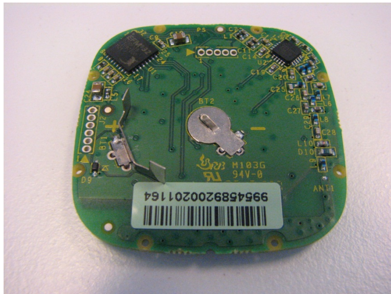
Photograph 9.2.2 Second side of the main PCB
