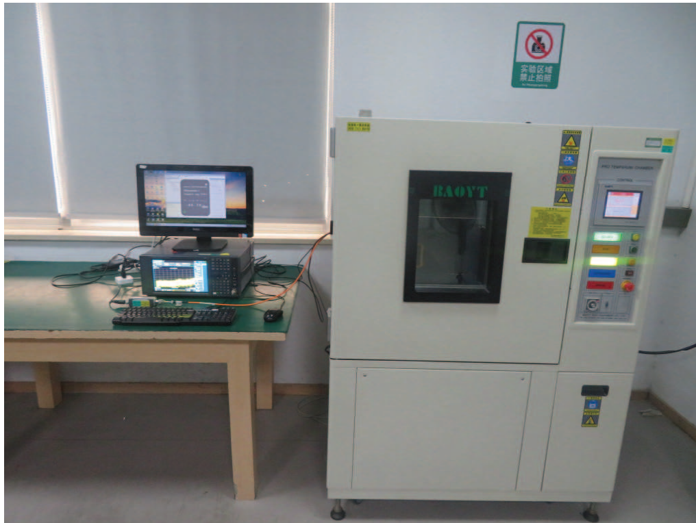
Photograph 2: Set-up for Conducted Test at Antenna Port
