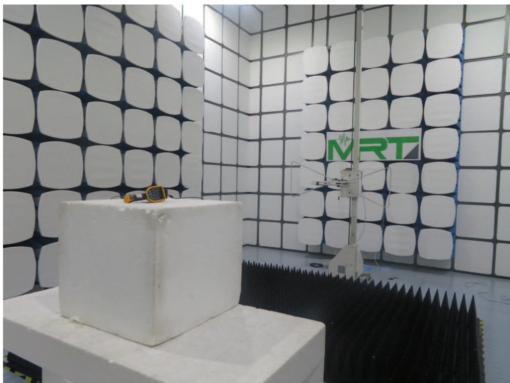
Photograph 5: Set-up for Radiated Spurious Emission, below 1GHz
