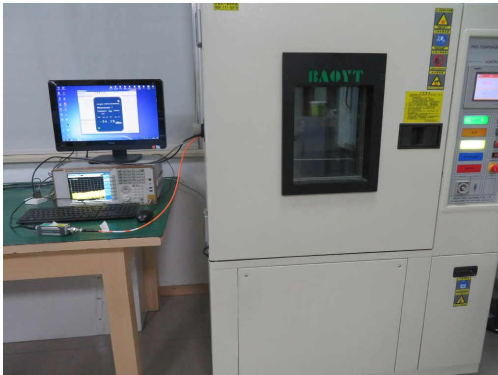
Photograph 2: Set-up for Conducted Test at Antenna Port
