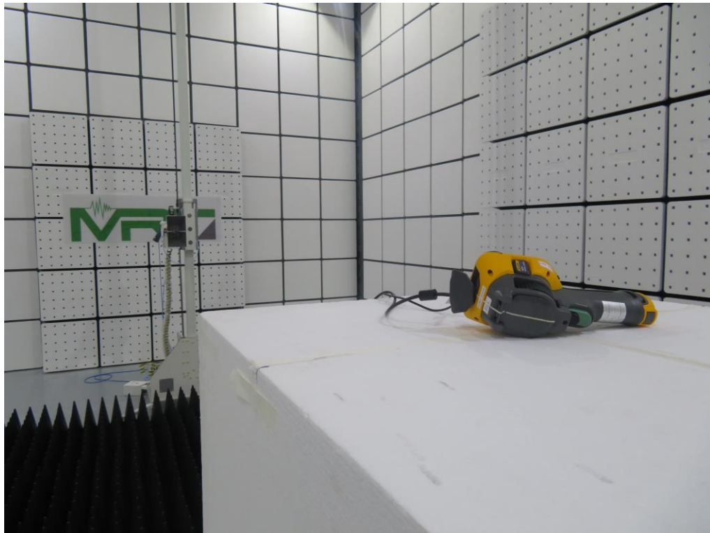
Photograph 6: Set-up for Radiated Spurious Emission, above 1GHz
