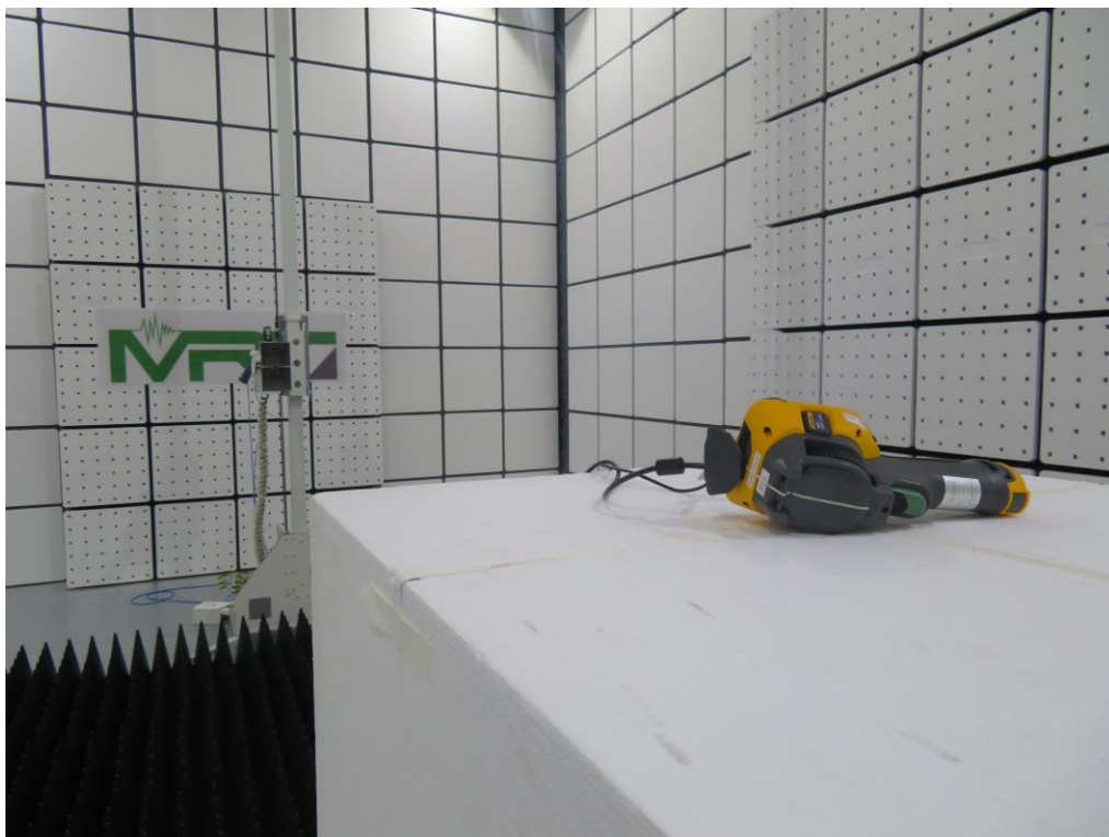
Photograph 5: Set-up for Radiated Spurious Emission, above 1GHz
