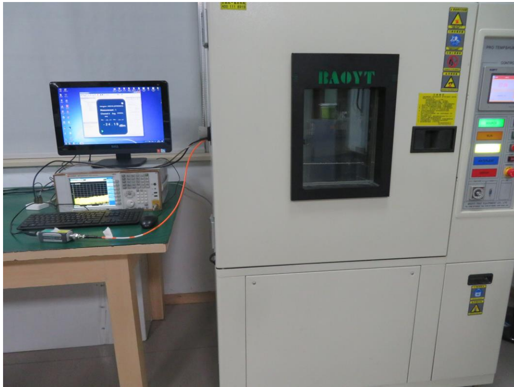
Photograph 2: Set-up for Conducted Test at Antenna Port
