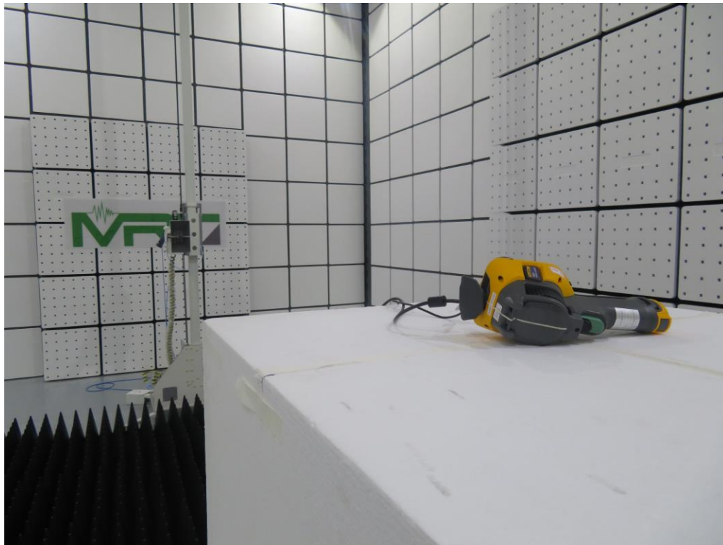
Photograph 4: Set-up for radiated spurious emission, 1GHz – 12.75GHz
