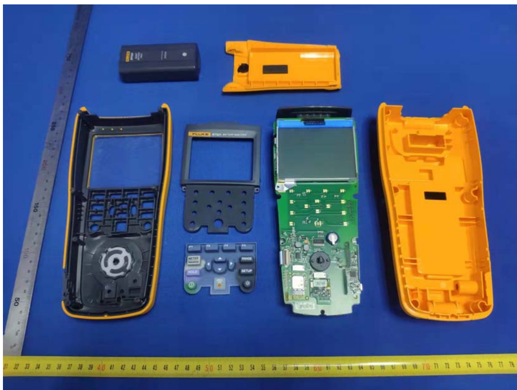
FIGURE 3 BATTERY ANALYZER (M/N: BT521) COVER REMOVED
