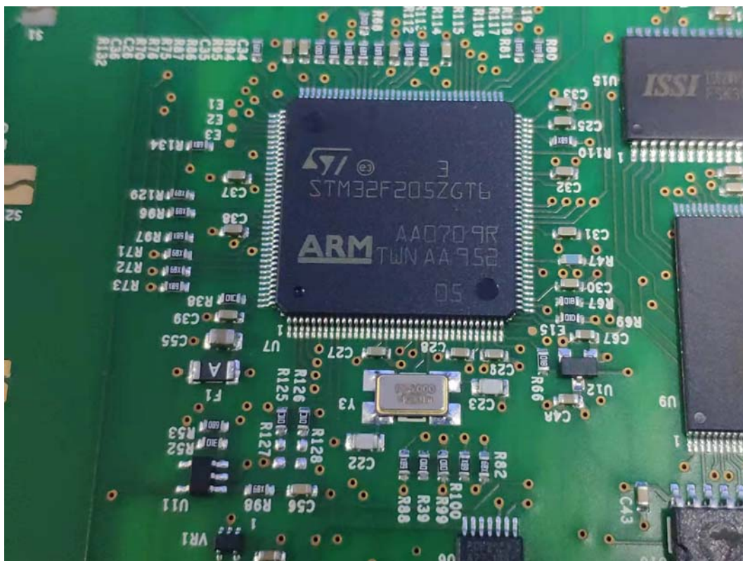
FIGURE 9 BATTERY ANALYZER (M/N: BT521) HIP & CRYSTAL ON MAINBOARD
