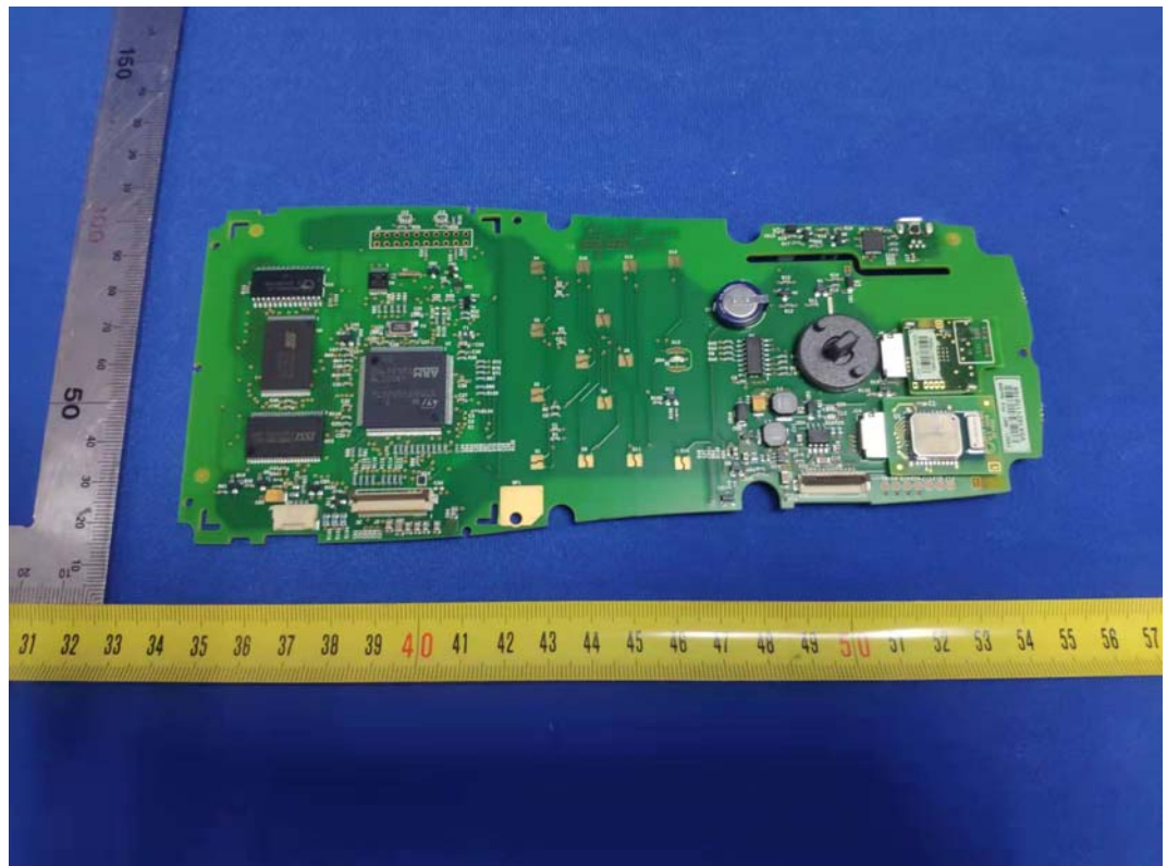
FIGURE 4 BATTERY ANALYZER (M/N: BT521) MAINBOARD FRONT
