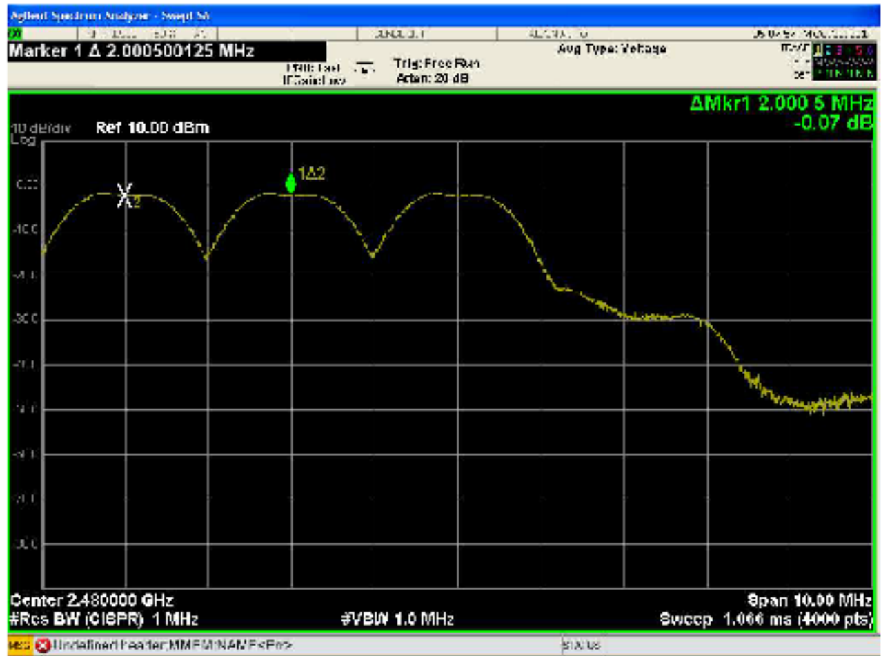
Figure 13: Channel Separation at 2480MHz
