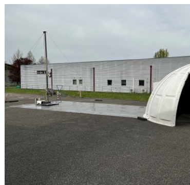
OATS Test setup (Biconic and Bi-Log antenna)
