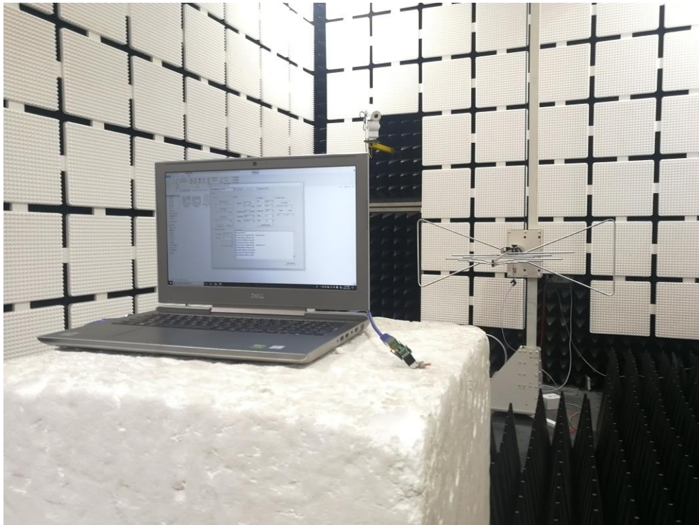
Photograph 3: Set-up for Radiated Spurious Emission, below 1GHz
