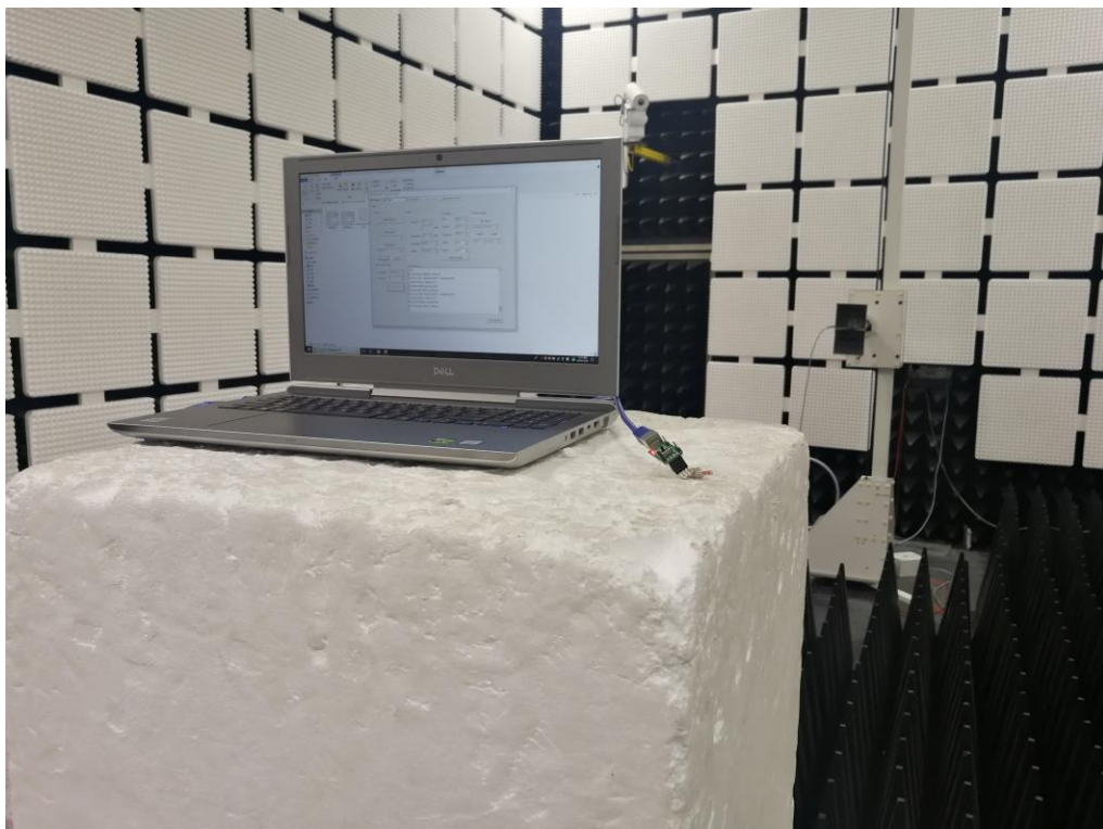
Photograph 4: Set-up for Radiated Spurious Emission, above 1GHz
