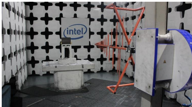
Radiated Setup 11 GHz – 40 GHz
