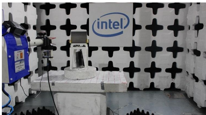
Radiated Setup 11 GHz – 40 GHz
