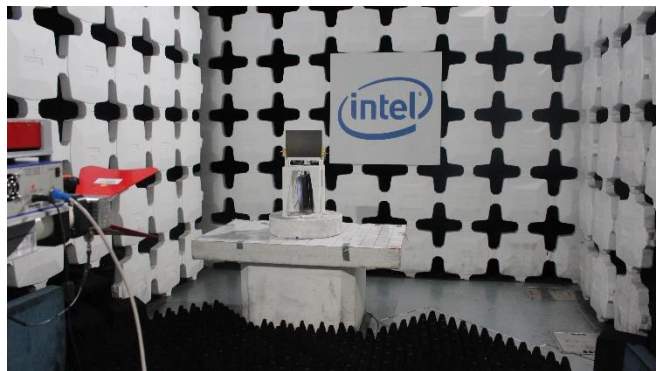
Radiated Setup 1 GHz – 11 GHz
