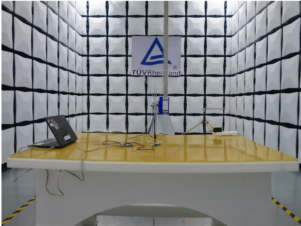
Photograph 1: Set-up for Transmitter & Receiver Spurious Emissions, Below 1GHz
