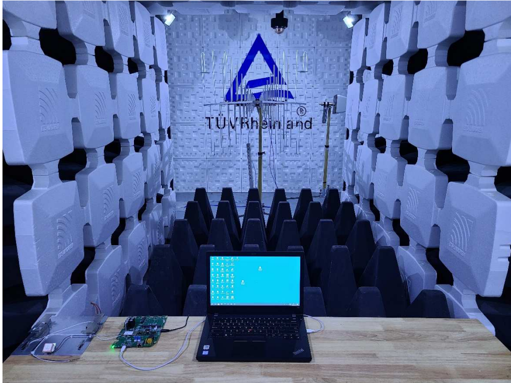
Photograph 7: Set-up for Radio Frequency Electromagnetic Fields (RS, 80MHz-1GHz)
