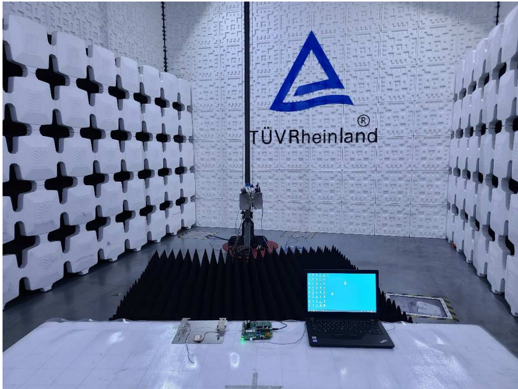
Photograph 5: Set-up for Radiated Emission, Above 1GHz
