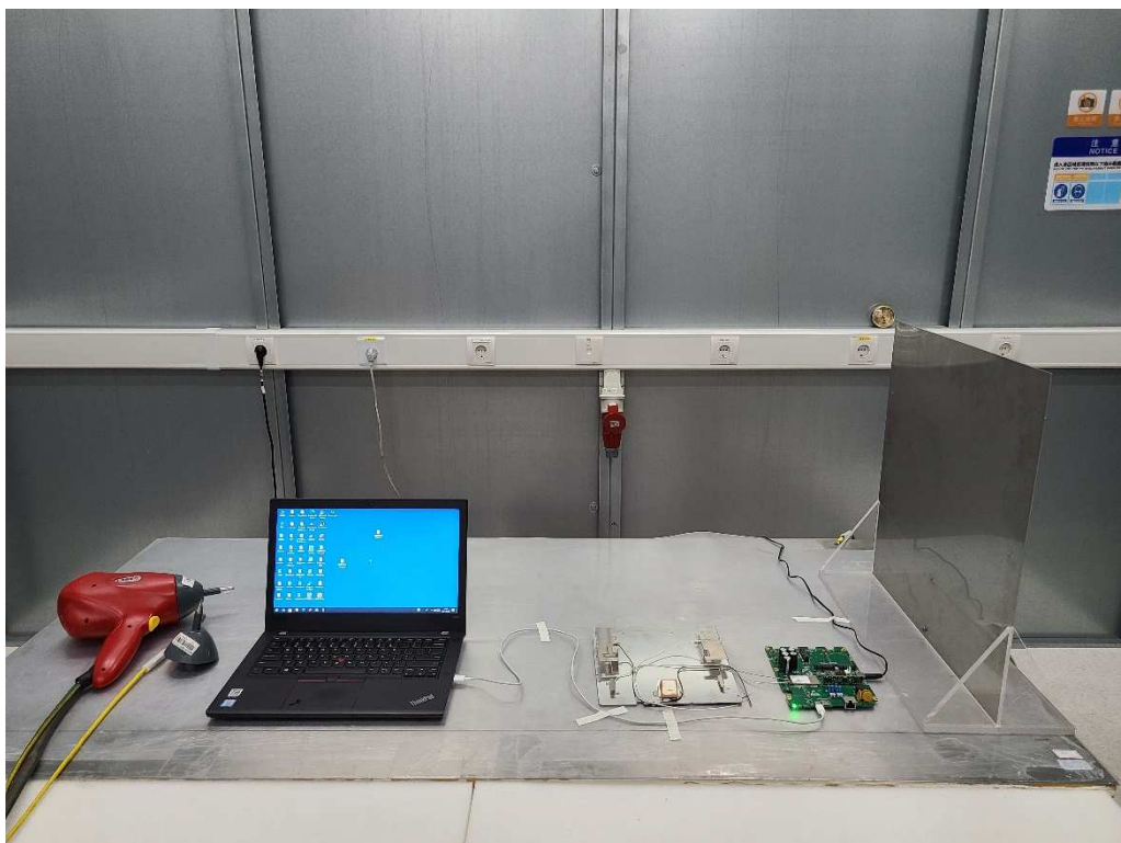
Photograph 6: Setup for Electrostatic Discharges (ESD)
